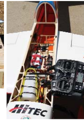
The entire upper forward part of the fuselage lifts off for access that dwarfs my Hitec Optic 6 Sport radio, used for this review.
