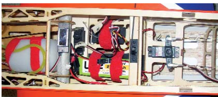
Hitec's HS-5665MH provides 122 ounce-inches of torque at 6 volts and 138 at 7.4. The entire aircraft is powered by a single LiFe Source Lithium-Iron-Phosphate battery from Hobbico. At 2100mAh and 6.6 volts, this 2-cell pack provides more than ample power for both flight pack and ignition module!
