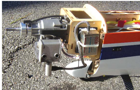
Fitting nicely under the cowling, the DLE 20 mounts to standard nylon beam mounts. Some modification is required to clear the motor box for the carburetor. Aeroworks has the DLE 20 mod kit available. It shows all the necessary steps to mount this little gasser.
