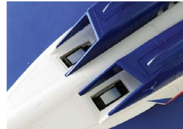
For cooling and balancing purposes, the two ESCs are mounted directly in front of the fans' intakes.
