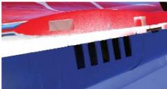
Under each wing root are vents to help exhaust the heat that builds up inside the nacelles.
