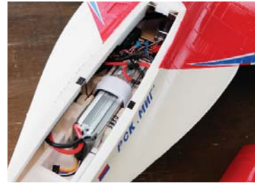
There's just enough room for the battery and radio components to fit in their designated area. Tucked inside in the aft area is the gyro.
