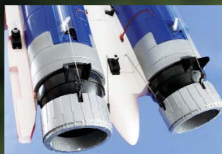
Here's a closer look at the servo set-up for the thrust vectoring.
