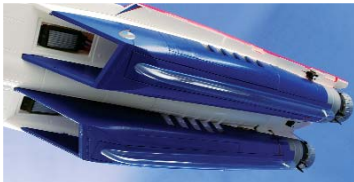
The bottom of each nacelle has clear plastic runners for smooth landings on grass fields.
