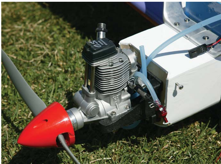
The World Models Groovy 3D, reviewed by Dave Keough in our May 2007 issue, uses an inverted O.S. 70 Surpass 4-stroke. This plane is typical of the many that would enjoy superior performance using the Uniflow fueling system. Yet this superior approach to "fuel plumbing" is not widely understood outside pattern and helicopter circles.
